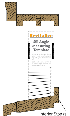
Fig. 15 Existing Window Frame - Side View
